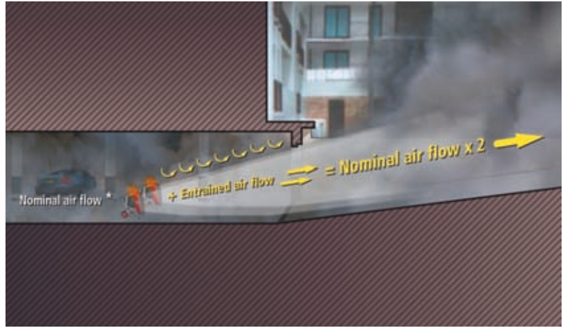
Fig 1 : 2 CarPark Fans in action
